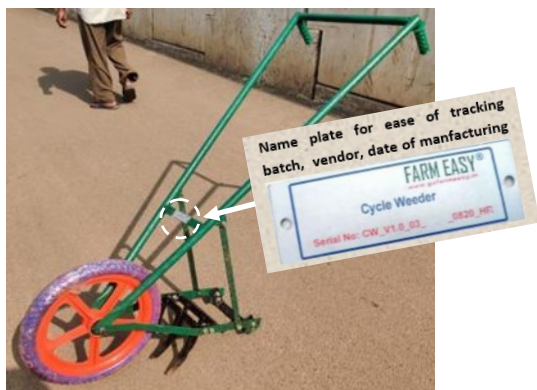
● Name plate for ease of tracking batch, vendor, date of manufacturing
